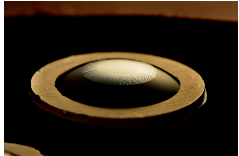
Ultrathin sheet (gray) at the top of a water miniscus (black) (courtesy of H. King)
