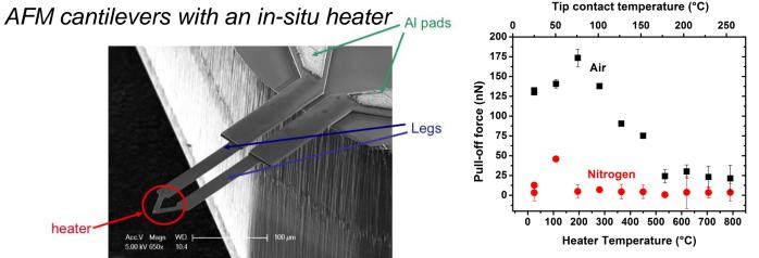
SiO<sub>2</sub> sample: In humid air, friction increases with temperature due to the thermal nucleation of a water meniscus, then decreases due to evaporation
