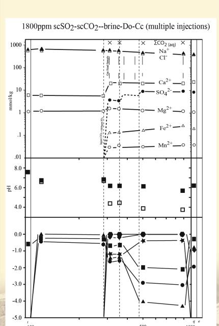
Hydrothermal experiment emulates carbonate reservoir (Madison Limestone).
