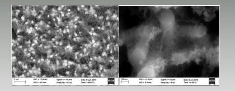
Successful fabrication of high Seebeck coefficient ZnO nanowires embedded in an aerogel matrix has been achieved. The nanocomposite decreases the thermal conductivity of ZnO nanowires by more than a factor of ten and has the potential to produce thermoelectric figures of merit greater than three.
