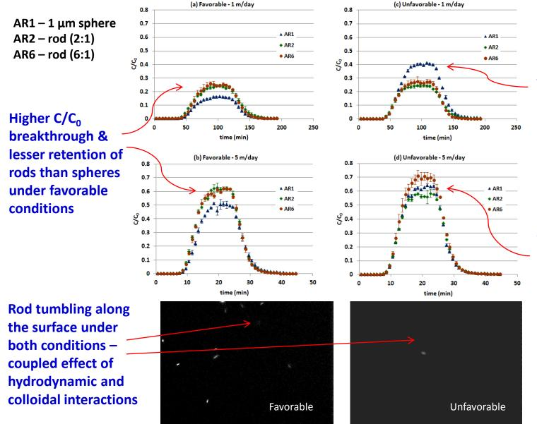
Lower C/C<sub>0</sub> breakthrough & greater retention of rods than spheres at low velocity under unfavorable conditions
