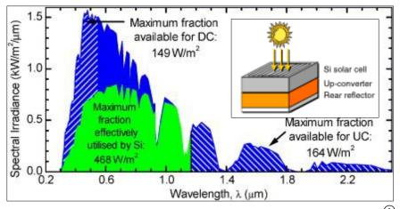
Our proposed idea of using RENs to harness the IR radiation in the solar spectrum.
