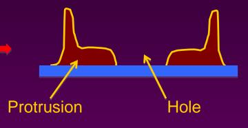
Vibration of complex fluids induces stresses that can cause protrusions, or in this case a "crown" with a hole at the center. This phenomenon may be directly relevant to the integrity of well-bore casings in oil production. The sample shown is a suspension of glass beads in water.
