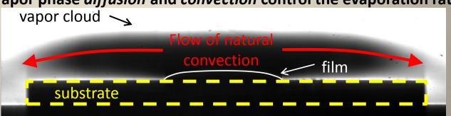
Correlation developed to compute the evaporation rate under combined diffusive and convective transport
