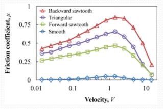
We showed that anisotropic surfaces can be used to regulate friction forces
