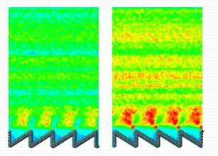
Friction forces are controlled by internal stresses arising in sliding polymer networks
