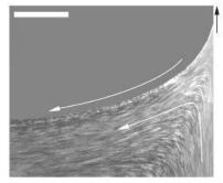
(a) c = 0.0. The small black arrow in the upper right hand corner indicates that the fluid near the substrate is carried into the film deposited on the moving substrate.
