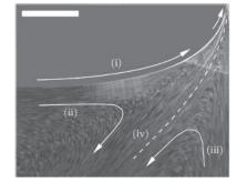
(b) c = 0.5. The small white arrow in the upper right hand corner indicates that fluid near the surface is swept into the film deposited on the moving substrate.
