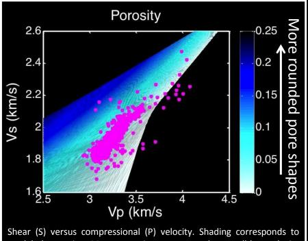
modeled porosity. Magenta points correspond to well-log velocity measurements within the Haynesville Shale. Porosity increases with darker colors as does the roundness of the modeled pore shapes.
