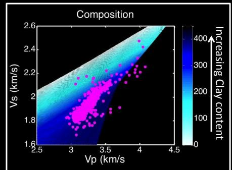
Shear (S) versus compressional (P) velocity. Points are measured data, and the color is composition number. Mineralogic composition includes quartz, calcite, kerogen, and clay. For increasing composition numbers, the clay content increases while the quartz and calcite decreases.
