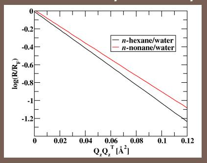
Direct comparisons with x-ray reflectivity experiments were made. Computational results show that alkane interfacial width increases with longer alkanes, in contrast to experiment.
