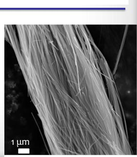
□ V₂o₅ nanowires have been prepared by hydrothermal treatment and vapor transport
