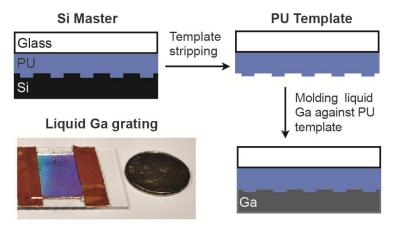
Combining **new nanofabrication methods**, we produced 1D liquid gallium (Ga) gratings, controlled the switching rates between liquid and solid phase transitions, and achieved high on/off contrast ratios of the surface plasmon polariton (SPP) resonances.
