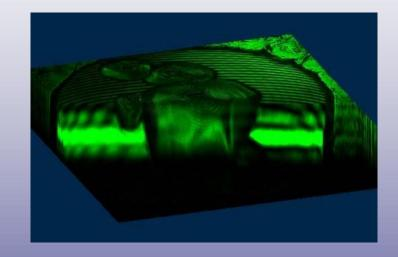
Above: Reconstructed image of pressureinduced freezing of water at room temperature
