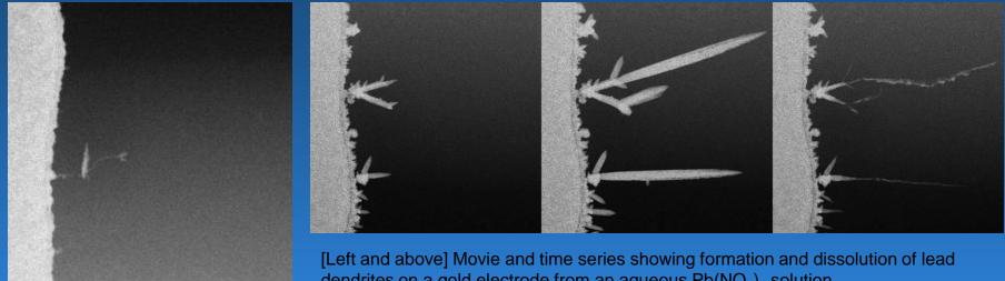
dendrites on a gold electrode from an aqueous  $Pb(NO_3)_2$  solution.
