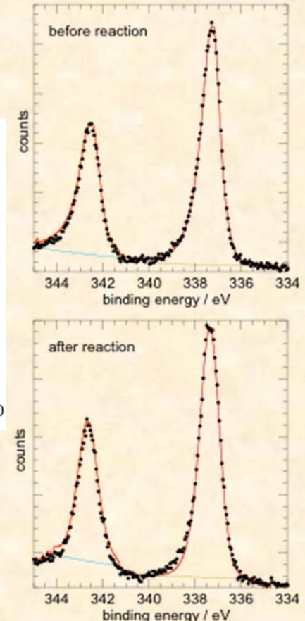
Despite their low surface areas, these materials are remarkably good oxidation catalysts. The oxide host stabilizes Pd(II) so well that there is no observable change in the state of near-surface Pd after reaction by XPS, and the lightoff profiles are so reproducible that kinetic parameters can be extracted from non-isothermal curvefitting.
