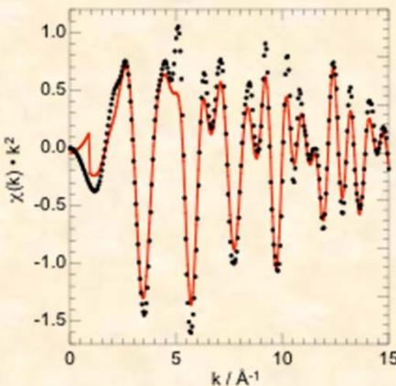
A family of Pd-containing complex oxides,  $\text{Ln}_2\text{BaPdO}_5$  ( $\text{Ln} = \text{La, Nd, Gd, Dy}$ ), was prepared and structurally characterized by powder X-ray diffraction and X-ray absorption spectroscopy. Pd(II) is incorporated into the structure as regular,  $\text{PdO}_4$  square planes.
