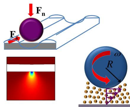
Analysis and experiment establish the stress level to damage a substrate. Our rheological theory predicts the normal and shear forces on a test particle in the flow illustrated; application of shear at or above the predicted threshold leads to wearpiece damage as seen below in before and after images (scale is 200 microns).
