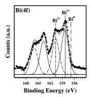
We performed XPS to study the oxidation states, curiously, we have discovered the Bi is in multiple oxidation states, +3 (55.6%) and +5 (44.4%). The crystallography is modeled as a +3 oxidation state. We are continuing our study of the structure by doing bond valence calculations and additional magnetic studies to confirm the mixed oxidation states.
