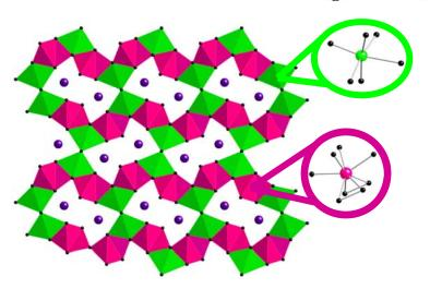
The structure consists of wave-like slabs of octahedral Bi (green) and bicapped trigonal prisms of La (pink) polyhedra. The potassium ions (purple spheres) sit inside of the channels made by the slabs.
