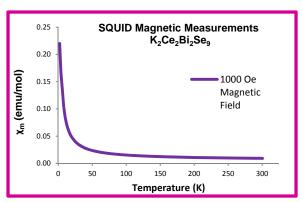
Magnetic susceptibility demonstrates the compound exhibits temperature independent paramagnetism where electrons have moved into the conduction band. The magnetic moment was determined to be 2.66 which is consistent with Ce<sup>3+</sup>. The XPS results suggest that the Bi is responsible for the delocalized electrons. These materials should be studied further for thermoelectric properties.
