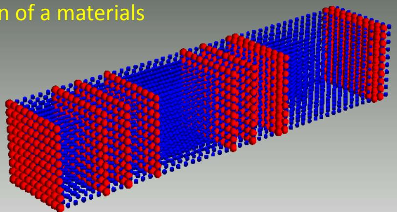
Random multilayer thin films offer the hope of tremendous reductions in lattice thermal conductivity through Anderson localization of phonons.
