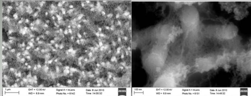
Successful fabrication of high Seebeck coefficient ZnO nanowires embedded in an aerogel matrix has been achieved. The material has the potential for thermoelectric figures of merit greater than three.
