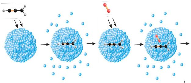
Helium nanodroplet isolation is used to trap and stabilize intermediates of prototype reactions that are central to combustion chemistry. Intermediates that result from the barrierless reactions between hydrocarbon radicals or between a hydrocarbon radical and molecular oxygen are being characterized with infrared laser spectroscopy. These studies add new chemical insight into the detailed mechanisms of reactions that are relevant to low-temperature hydrocarbon oxidation and soot formation.
