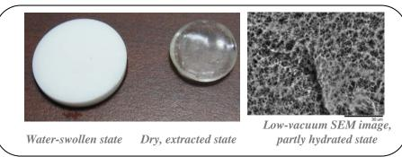
Gels were swollen in  $D_2O$  and characterized by ultra-small angle neutron scattering (USANS) using the BT5 Perfect Crystal Diffractometer at the NIST Center for Neutron Research.
