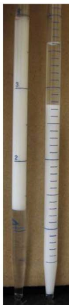
emulsions stabilized with surface coated nanoparticles (L) oil-in-water; (R) water-in-oil
