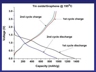
In this project, we prepared and tested tin oxide and tin based compostie anode films with a variety of porous morphologies using Electrostatic Spray Deposition (ESD) technique. Material characterization and electrochemical analysis were conducted. This research has significantly enhanced our understanding of fundamental issues regarding intrinsic properties of porous tin oxide and tin based composite materials as high performance anodes for Li-ion batteries.
