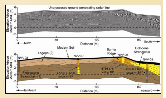
Raw (top) and processed (bottom) ground-penetrating radar lines from Navegantes. The features shown are interpreted as the mid-Holocene highstand ridge, emplaced upon the underlying Pleistocene (~120,000 years old) regressive strandplain. A radiocarbon date at the base of the ridge indicates that this ridge is of mid-Holocene age, at the approximate time of the sea-level highstand identified along the southern Brazil coast.
