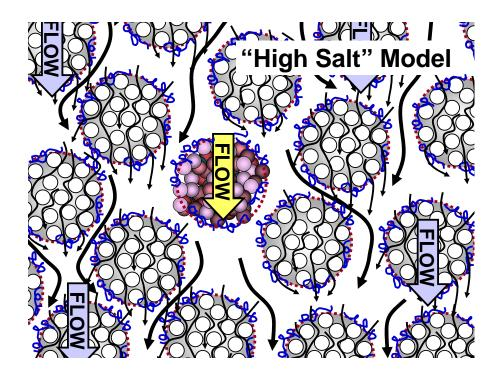
Schematic diagram of a bed of silica gel composite particles immersed in aqueous solution with sufficient salt so that ionic double layers can be expressed within the very fine pore spaces
