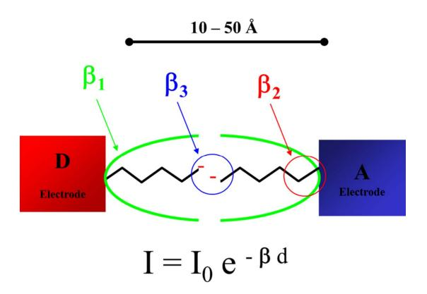
Tunneling conductivity of carboxy-terminated SAMs depends critically on pH
