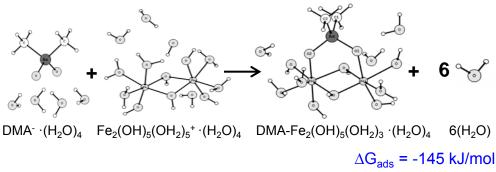
Example DFT/B3LYP calculations on the formation of the thermodynamically most stable DMA complex with iron clusters
