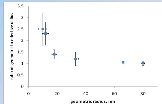
Plot of ratio of geometric to effective radius over the geometric radius of nanometer-sized electrodes.
