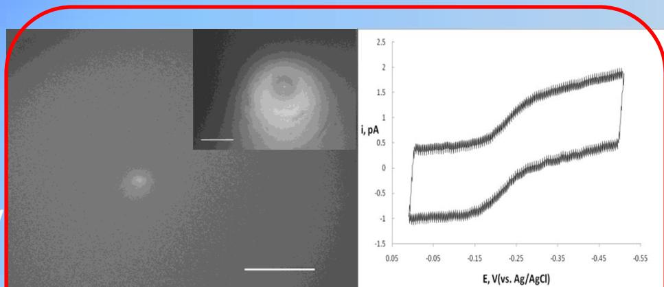
Geometric radius measured from scanning electron microscopy images is  $12.5 \pm 2.1$  nm. Effective electrode radius measured from cyclic voltammogram is  $5.4 \pm 0.7$  nm.
