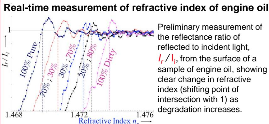
We have applied our new model toward a first real-time measurement of refractive index changes in auto-engine oil of slightly varying states of degradation. By contrast, in the auto industry, oil quality is “monitored” by mileage-based software without any actual sensing.
