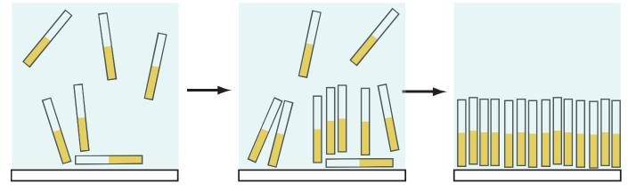
Schematic of the assembly process. As nanowires deposit from solution, they diffuse across the surface and rotate perpendicular to it. With increasing numbers of neighbors, "standing" particles become stabilized and form a columnar array.
