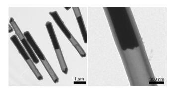
Transmission electron micrographs of partially etched nanowires. The black segments are Au with the lighter gray being a silica coating. The small dark ends of the wires are Au caps to prevent premature etching.
