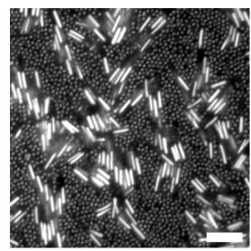
Inverted optical reflectance micrographs showing assembled nanoparticles on an open surface (left) and within a microwell (right). Points indicate standing wires; lines indicate laying wires. Scale bar is 5 µm.
