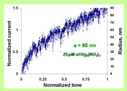
Growth of a Hg nucleus on a 90 nm Pt electrode. Experimental current transient (symbols) is fitted to the theory (solid line).
