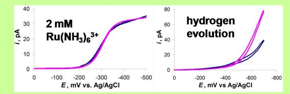
Electrodeposition of a small Pt cluster at a 65 nm Au electrode. The voltammograms of  $\text{Ru}(\text{NH}_3)_6^{3+}$  obtained before (blue) and after (pink) the deposition are essentially identical (A), but hydrogen evolution voltammetry shows the formation of a Pt cluster (B).
