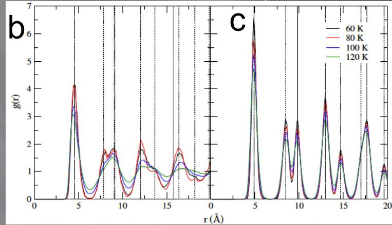
**$\text{CF}_4$  on Hydroxylated  $\alpha$ -quartz:** Figure (d) below shows the first layer of the  $\text{CF}_4$  film and the top layer of the  $\alpha$ -quartz substrate. Figure (c) shows the corresponding 2-D radial distribution function,  $g(r)$ .
