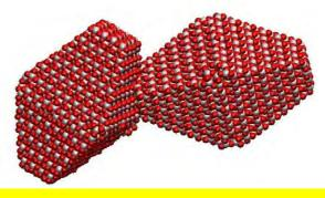
TiO<sub>2</sub> (anatase) nanoparticles aggregate preferentially on the edges of {001} facets and the edges between two {101} facets.
