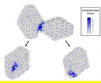
Electrostatic forces dominate and are the highest between aggregating edge atoms.
