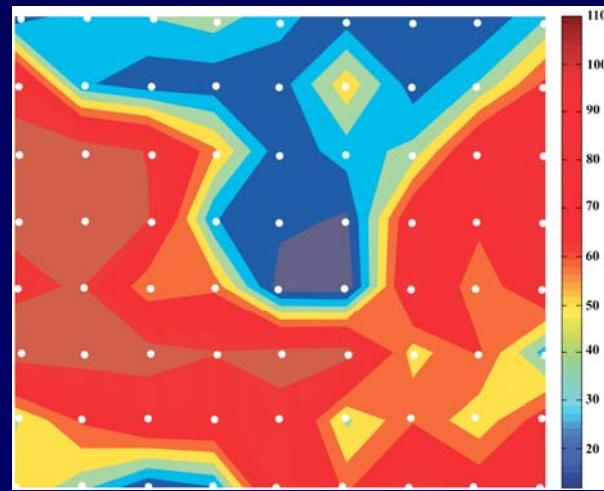
Young's modulus map (left) and bulk modulus map (right) of the area of interest. Organic matter (dark blue) is characterized by low (10-15 GPa) values of Young's modulus as well as low (5-10 GPa) values of bulk modulus. The bar on the right is in GPa. Sampling area is  $120 \times 110 \mu\text{m}$ .
