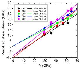
Hardness and yield stress are linear with friction (shear strength) of grain boundaries
