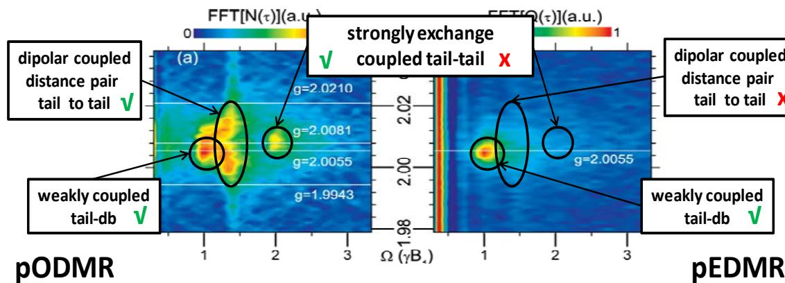
Plots of the optically (a) and electrically (b) detected recombination rate as a function of the magnetic resonance induced spin-Rabi nutation frequency  $\Omega$  and the  $g$ -factor of the recombining charge carriers. The measurements were conducted on identical a-Si:H films and under identical conditions.
