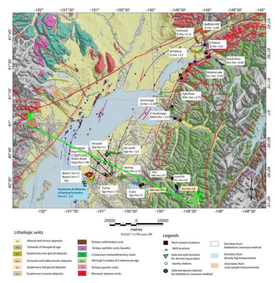
We have collected gravity observations in subregions to estimate variations in nearsurface densities (white boxes). These are comparable to estimates from well logs (blue boxes) or surface samples (tan boxes). Geology/gravity cross section (green line) shown in next slide.
