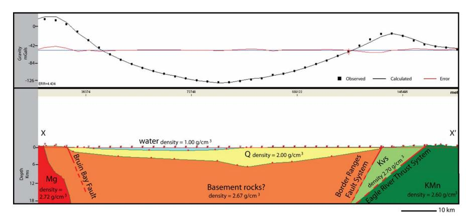
Cross section along X-X' (see previous slide) showing observed gravity (black dots), calculated gravity (black line) and error (red line). Preliminary geologic/density model shown below. Model is based on well log, seismic reflection, surface geology and other information.
