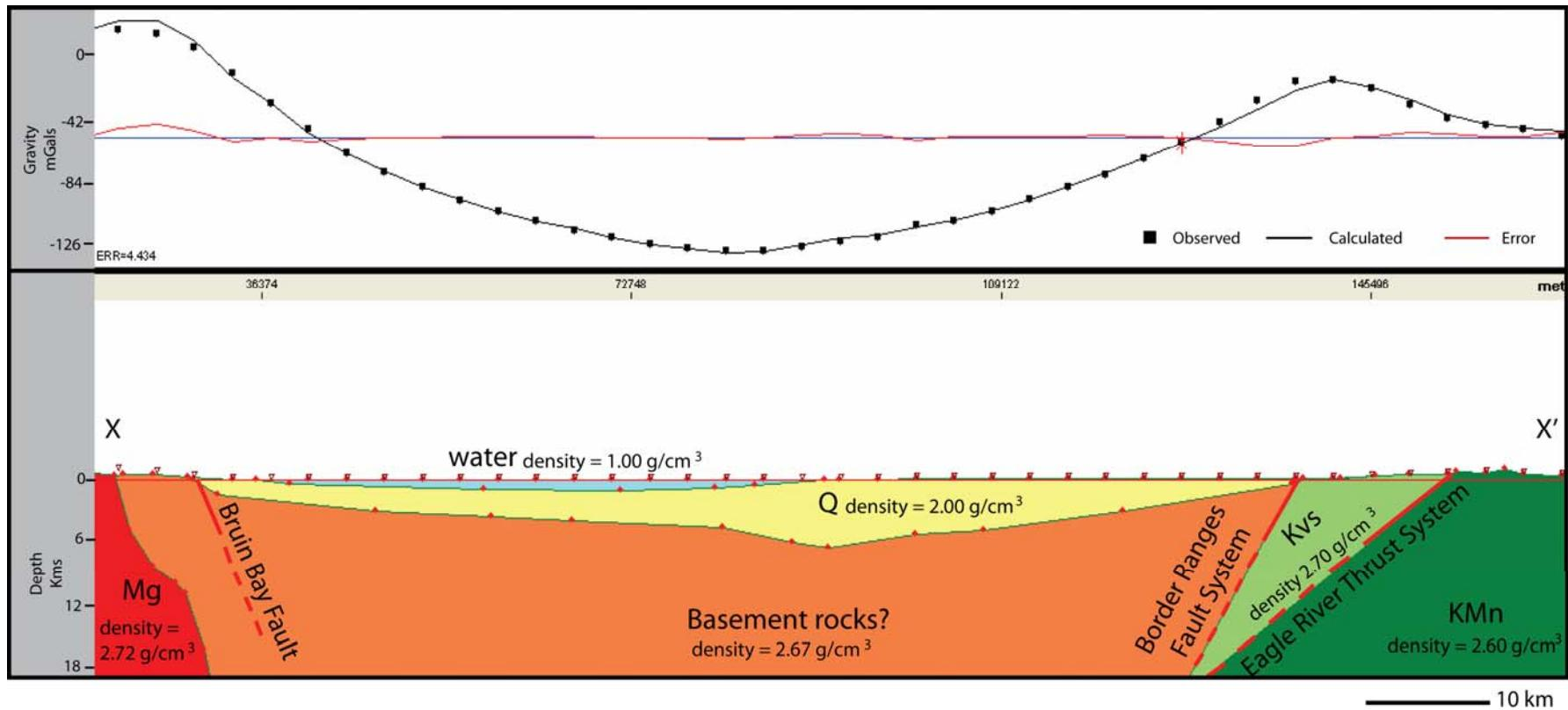
Cross section along X-X' (see previous slide) showing observed gravity (black dots), calculated gravity (black line) and error (red line). Preliminary geologic/density model shown below. Model is based on well log, seismic reflection, surface geology and other information.
