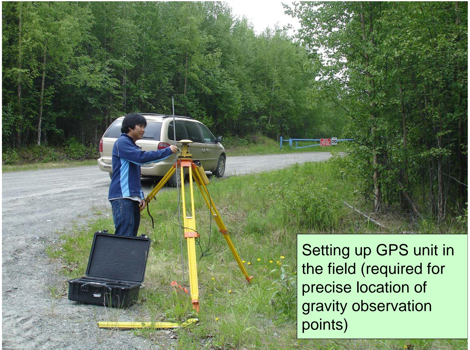
Setting up GPS unit in the field (required for precise location of gravity observation points)
