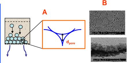
(A) Schematic of formation of latex composite membranes (LCM) by filtration of colloidal particles. The interstitial spaces between the particles serve as narrow dispersed pores for size separations. (B) Scanning Electron Micrograph of a LCM (top and bottom views) of 0.62  $\mu$ m particles.
