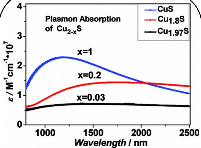
Tunable plasmonic absorption spectra of  $\text{Cu}_{2-x}\text{S}$  nanocrystals prepared from a sonoelectrochemical approach.
