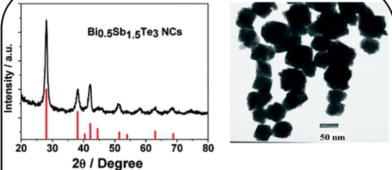
High quality tertiary thermoelectric nanocrystals prepared by a wet chemistry approach.
