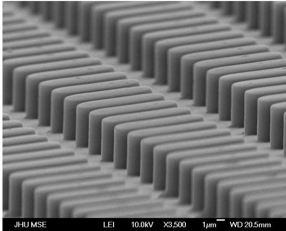
We study the transport of suspended colloidal particles in micromodels of porous media. In the picture, we can see an ordered array of PDMS *obstacles* in which we study the effect of anisotropic structures (media) on the diffusive and convective transport of finite size particles.
