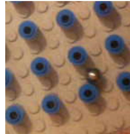
We also investigated macroscopic transport in periodic systems to understand the differences and similarities with the phenomena observed at the microscale. The picture shows the motion of a sphere through an ordered array of cylinders. Directional locking was observed in these experiments in excellent agreement with our theoretical predictions and numerical results.
