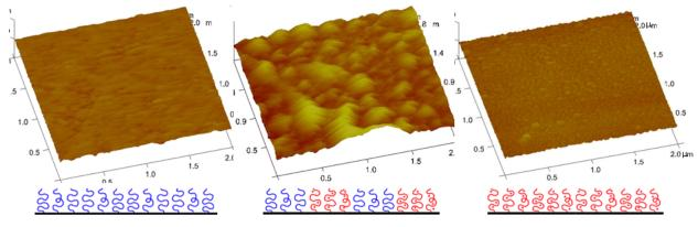
In preliminary experiments, we discovered that in this mixed brush system, the chemical dissimilarity between the two species results in the formation of microscopic phase-separated structures.
