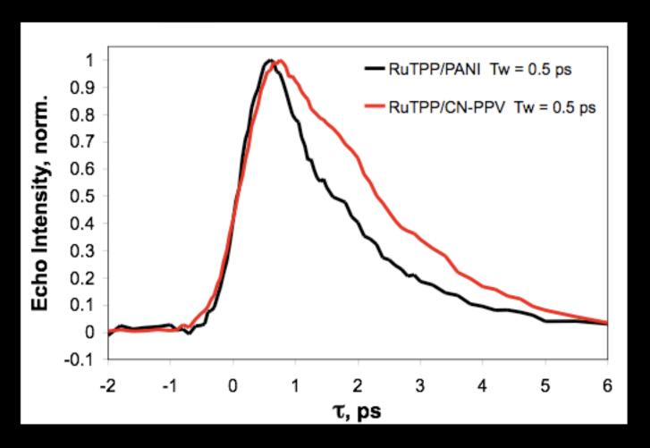
Different vibrational echo decays are evidence of different dynamical processes, which we will relate back to material function.
