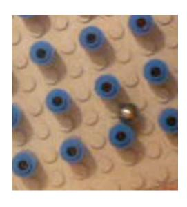
We study the transport of suspended colloidal particles in micromodels of porous media. In the picture, we can see an ordered array of *obstacles* in which we study the effect of anisotropic structures on the diffusive and convective transport of finite size particles.
