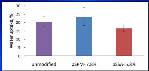
water uptake for sintered membranes after soaking in water at room temperature for 24 hours.
