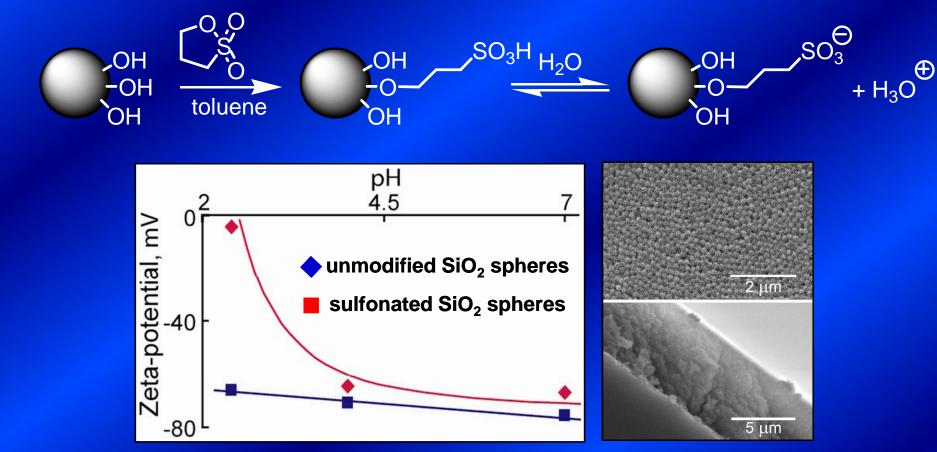
sulfonated silica spheres can be self-assembled into colloidal films
