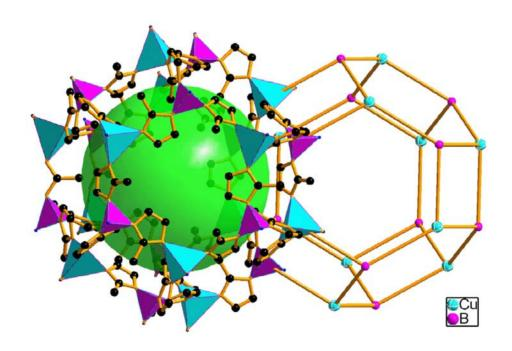
Sodalite Cage based on Cu-B Imidazolate
