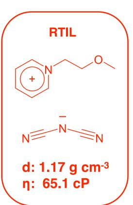
Room temperature ionic liquids (RTILs) such as the methoxyethyl-pyridinium/ dicyanamide (shown at left in red) are becoming widely used for electrochemical, enzymatic, and fuel cell applications.
