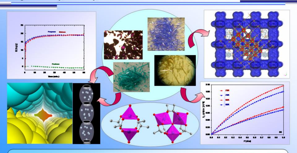
We have designed and synthesized four types of microorous metal organic frameworks (MMOFs). By modifying the metal building units and ligands we have successfully optimized pore volume and surface area to reach a high hydrogen uptake of 2.1 wt% (77K, 1 atm) and 4.0 wt% (77K, 40 atm), placing these materials among those with the highest values reported thus far.
