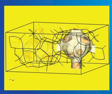
The wire frame above shows the zeolite's atoms framework within one unit cell. One of its pores is highlighted. In white are the locations within the zeolite's s pore that are available to the gas molecules, while the preferred sites are in orange.
