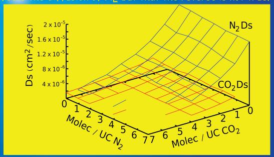
The 3D plot below shows Self Diffusion for  $CO_2$  and  $N_2$  mixtures within ITQ-3. Note how  $CO_2$  (in red) diffuses more slowly than  $N_2$ , and its concentration greatly affects the behavior of the faster  $N_2$  molecules.
